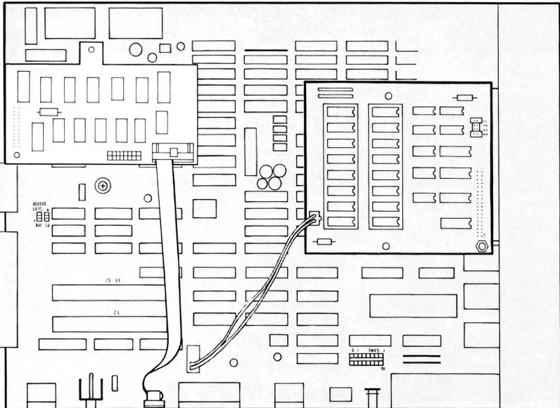
*Reference Manual*, pages 1-19 through 1-20. When the computer is open, locate the RGB connector on the right side of the main board.
