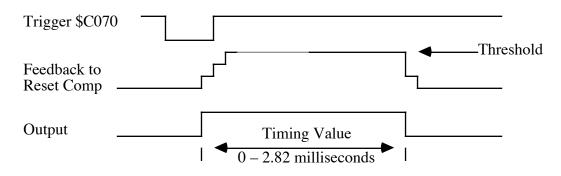
Figure 3–Paddle Circuit Recharge Timing
