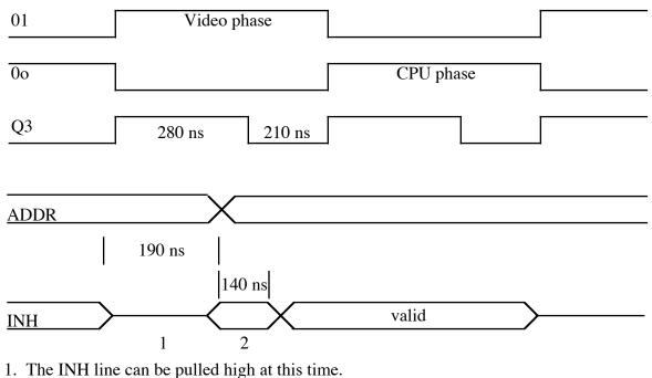
The INH line can be pulled low (or high) after the addresses are valid at 190 ns, but before 300 ns (from 0o).
