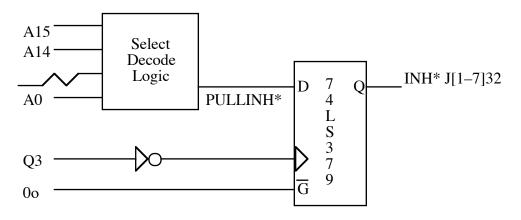
Figure 2–Circuit Implementing /INH Function
