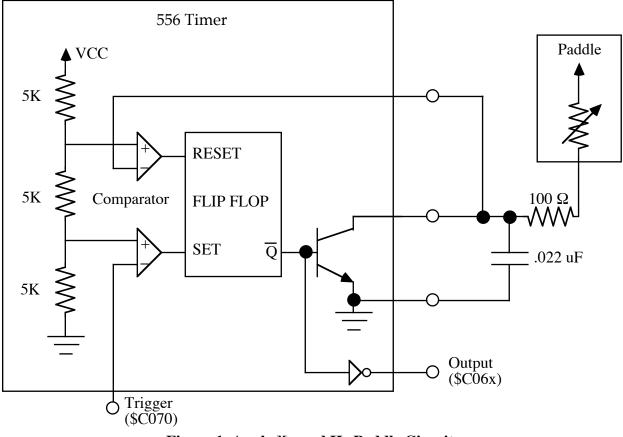
Figure 1–Apple ][+ and IIc Paddle Circuit
