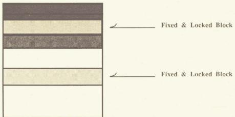
Fortunately, part of the Memory Manager's job is reorganizing memory blocks. It shuffles movable blocks around in an efficient and resourceful manner. This is done by removing blocks that are flagged as unused and then sliding blocks around in order to fill any gaps. The effect is that the landscape inside the computer is kept neat and orderly.
