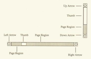
The scroll bar is the most complex type of control you can define. The Window Manager uses scroll bars in windows to scroll an area of data. However, if you want to put a scroll bar into a dialog box just to see what it's like, you'll need to know the information provided by Table 11-8.
