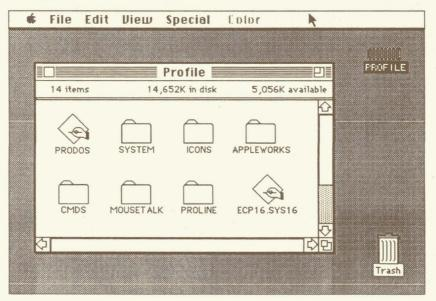
It is the responsibility of the Event Manager to track the location of the mouse and update the mouse pointer on the screen. The mouse pointer, an arrow shape, marks the position on the screen where the mouse is located on the DeskTop. Moving the physical mouse device will cause the mouse pointer to move accordingly on the screen. This function is completely transparent to the DeskTop application because it relies on the interrupt feature of the Apple IIGS microprocessor.
