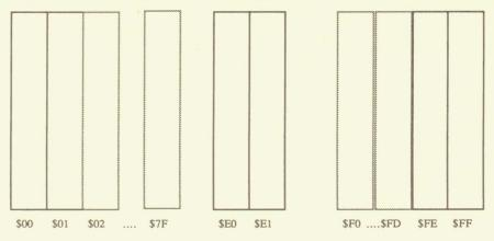
Each memory address (location) in the computer's RAM is represented by a bank number and an offset within that bank. For example, address \$000200 indicates memory location \$0200 in bank \$00, the first bank of memory. Memory location \$00A8 in bank \$E1 is expressed as \$E100A8. The first byte value represents the bank number; the second word value indicates an offset within that bank.
