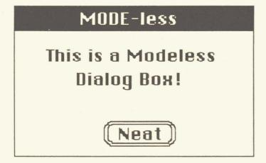
A good example of a modeless dialog would be a spelling checker in a desktop word processor. The modeless dialog can display a misspelled word and offer a suggestion for the correct spelling. In response, you can edit the text in your document window, then click a Next button inside the modeless dialog box to go to the next misspelling.
