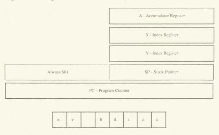
The 6502 chip used in older Apple II machines can only handle eight-bit operations.
