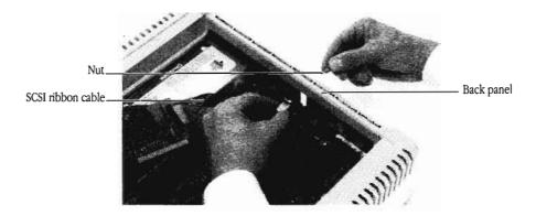
Figure 1-5 Connecting the ribbon cable
