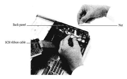
Figure 2-4 Connecting the ribbon cable
