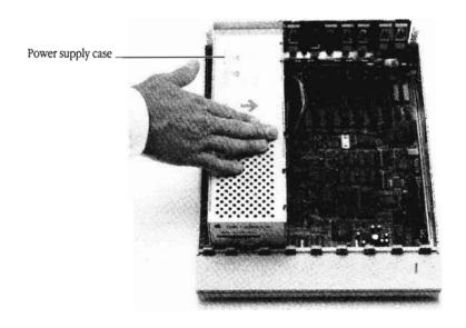
Figure 2-3 Touching the power supply case
