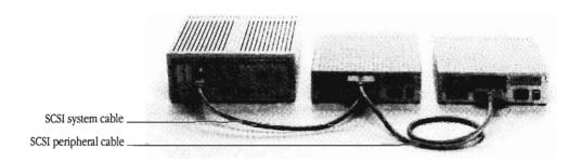
**Figure A-6** Connecting the peripheral cable (without cable extender)
