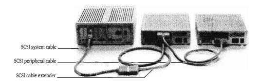
Figure A-7 Connecting the peripheral cable (with cable extender)
