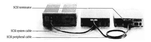
**Figure A-8** A completed chain (without cable extender)
