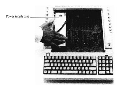
Figure 1-3 Touching the power supply case
