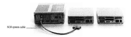
**Figure A-3** Connecting the system cable
