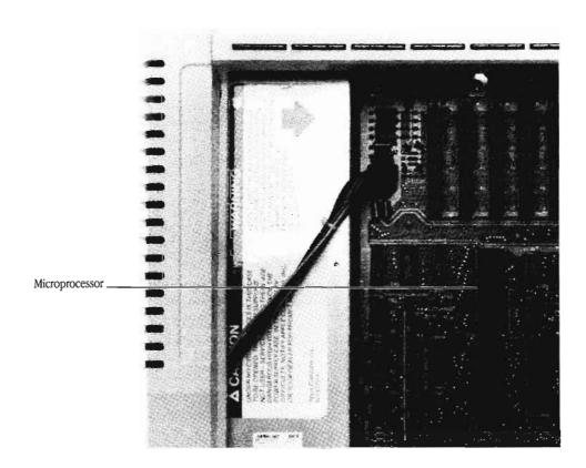
Figure 1-4 Locating the computer's microprocessor
