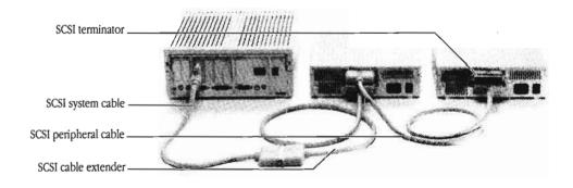
Figure A-9 A completed chain (with cable extender)
