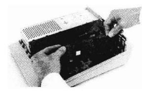
Figure 2-5 Inserting the card in the slot
