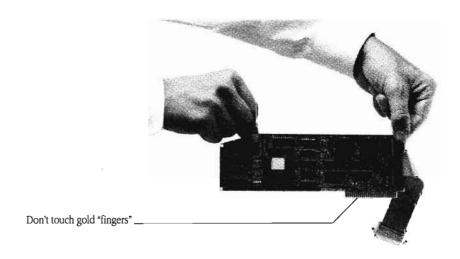
Figure 1-2 Handling the card carefully
