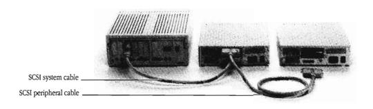
Figure A-4 Connecting the SCSI peripheral cable (without cable extender)
