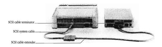
Figure 1-10 The completed connection (with cable extender)
