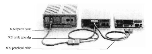
Figure A-5 Connecting the SCSI peripheral cable (with cable extender)
