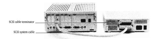
**Figure 2-8** The completed connection (without cable extender)
