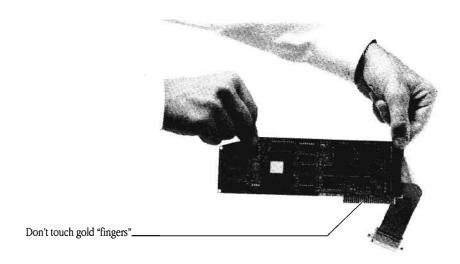
Figure 2-2 Handling the card carefully
