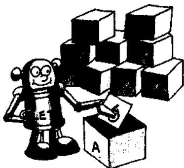
**LET** tells the computer to label a section of its memory and put a particular value in it e.g. `LET A=6` means label a section of memory "A" and put the value 6 in it. "A" is called a "variable" and putting something in it is called "assigning a value to a variable".
