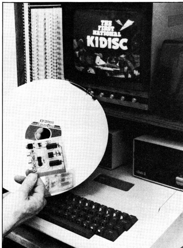
Interface to a laserdisc.
