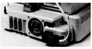
**THE FAN** also filters out surges and spikes in the main supply which can damage your hardware and corrupt data. A single switch ensures that all peripherals are turned off at the same time as the *Apple*.
