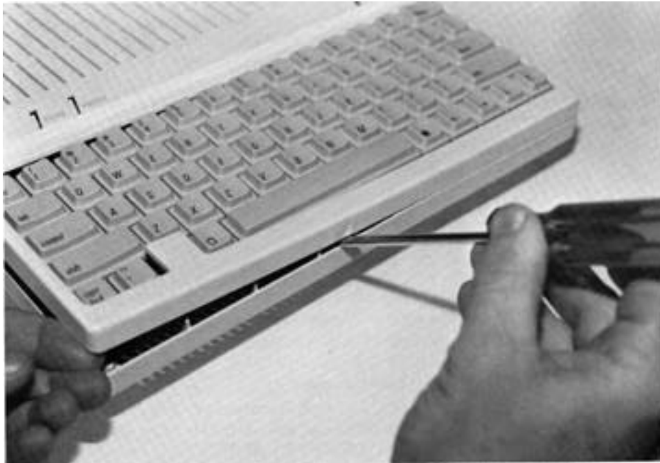
Figure 1-4. Releasing the //c keyboard bezel snap
